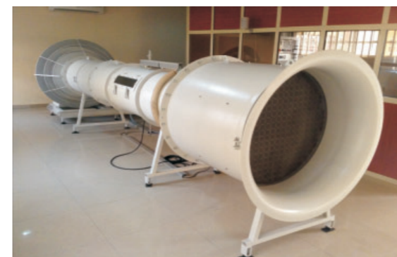
Wind tunnel for testing & calibrating wind instruments
